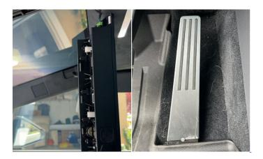
A Cybertruck owner shared photos of his vehicle's gear selector hanging by a wire. A former Tesla engineer told DailyMail.com that this issue will keep happening, due to an engineering flaw in the vehicle design. The Cybertruck also
